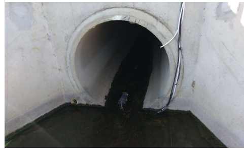
Pump with plumbing to autosampler, flow meter and depth sensor install in the inlet pipe
